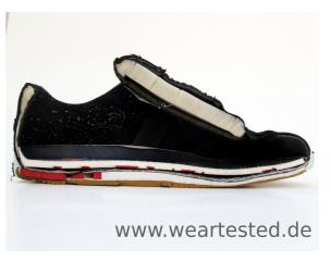
landings and bails. Although at first sight, the red foam doesn't differ too much from the white parts, it does seem to absorb shocks better and doesn't bounce back as much, so the XLK sole does its job pretty well. The thicker insole provides further cushioning and, together with the new sole construction, the Mike Mo turned out to be an adequate model for high-impact skating.
